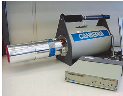
A multi-channel analyzer that can detect whether uranium has been enriched (Dean Calma/IAEA).
